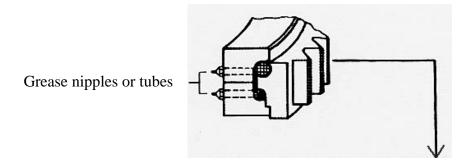
THE BEARING is to be greased with KRØLL lubricant no. 3 after every 20 hours' operation or, alternatively, a minimum of once a week, unless the crane is fitted with a automatic greaser unit.
